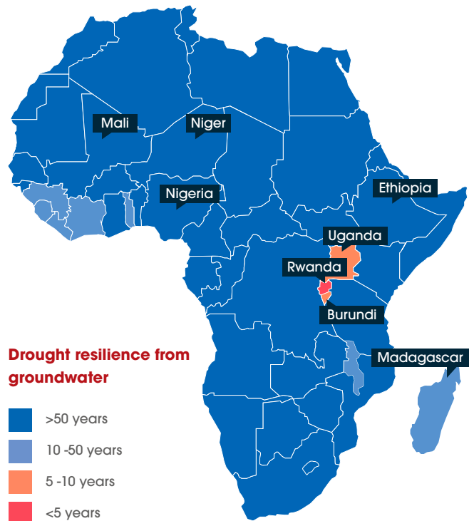
Years of reserves of potentially usable groundwater at a national level, based on current usage plus current population using 130 litres per person per day, assuming no active recharge
